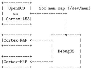
NOTE: Firewalls are configurable in K3 SoC and depending on various types of device configuration, this function may be blocked out. Typical behavior observed in such cases is a firewall exception report on the security controller and armv8 processor reporting a system error.
